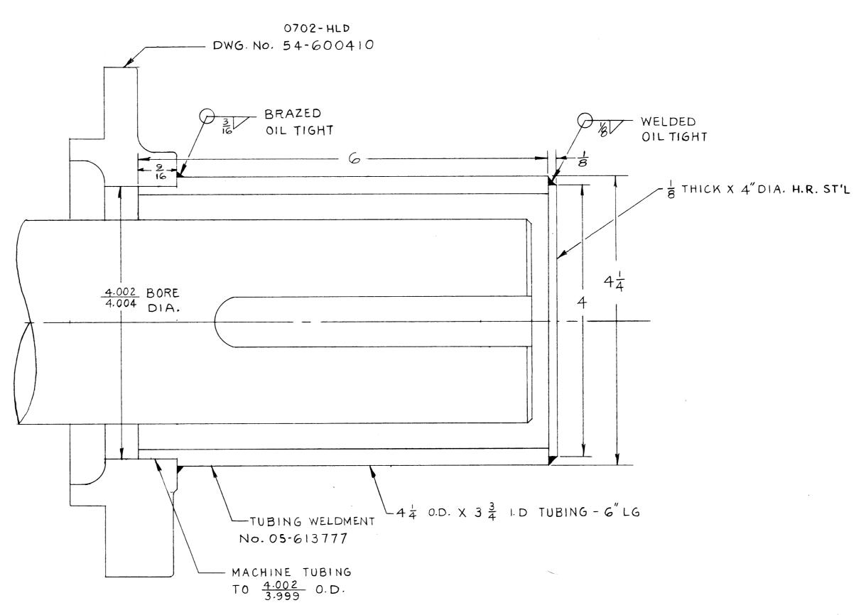
NOTE: SHAFT GUARD — 0702-HLD-85-100097 CONSISTS OF THE FOLLOWING PARTS: 1-COVER-BRG-L.S.-OPEN-54-600410 I-TUBING WELDMENT NO. 05-613777
