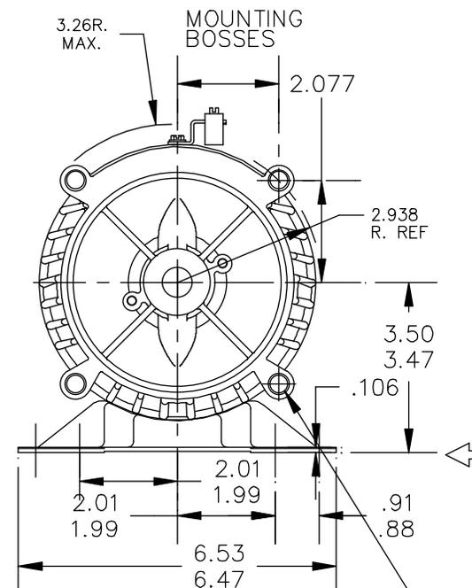
ECCENTRICITY OF THIS SURFACE (WITH INDICATOR MOUNTED STATIONARY RELATIV TO SHAFT) MUST NOT EXCEED .004 T.I.R.
