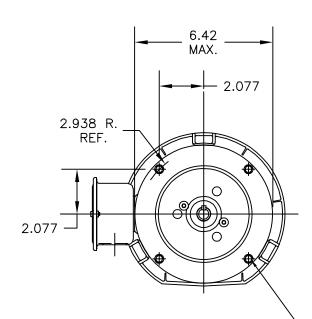
.375-16 UNC-2B (4 HOLES) .70 MIN. FULL THREAD THESE HOLES FIT A GAGE HAVING A RABBET 4.5005 DIA. AND 4 PINS .2917 DIA. LOCATED ON THE BASIC HOLE POSITIONS.
