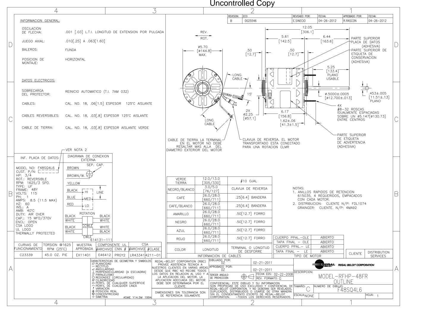
Uncontrolled Copy 4 批准 ECO E.SINECIO R.RASCON 0025546 04-26-2012 04-26-2012 12.05 [306.1] 5.61 6.44 ROT. [142.5] [163.6] ø5.70 .50 [12.7] [ø144.8]-[12.7] MAX. 5.25 [133.4] 453±.005 ø.5000±.0005 15° [ø12.700±.013] [11.51±.13] 2X 6.17 Ø2.25 [156.8] [ø57.1] 1.62±.06 [41.3±1.5] SEP. CAP. MODEL NO: F48SQ4L6 CUST. P/N: HP: 3/4
